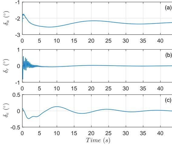
Figure 8: Panel (a), (b), and (c) show the evolution of the deflection of the control aerodynamic surfaces.
