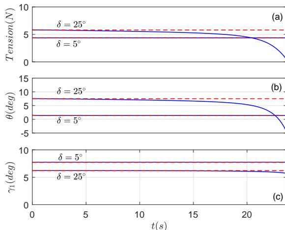
Figure 5: Panels (a) and (b) show the evolution of the tether tension, kite pitch angle and elevation angle, respectively for two reel-in maneuvers with  $(\delta, v_{in}) = (5^\circ, -0.064)$  and  $(\delta, v_{in}) = (25^\circ, -0.05)$
