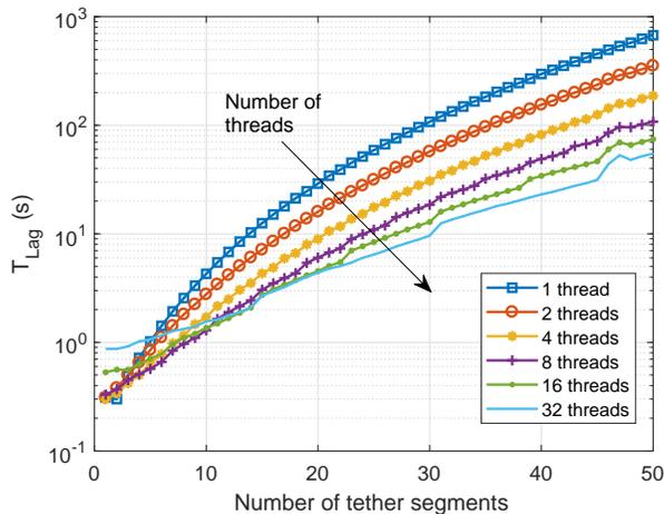
Figure 2: Computational time versus number of tether segments.
