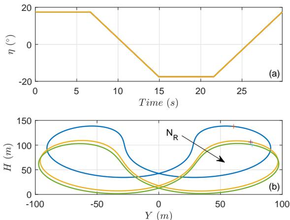
Figure 6: Panel (a) and (b) show the control law for  $\eta$  and the trajectory of the center of mass of the kite, respectively.
