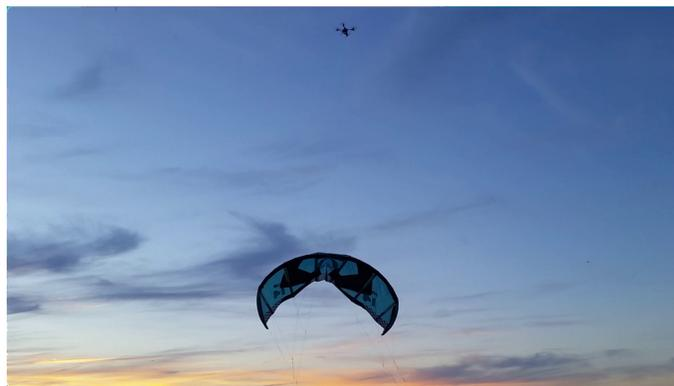
**Fig. 1 Custom made drone launching a 9 m<sup>2</sup> kite. Photo credits: Marcos Jerez Venegas.**
