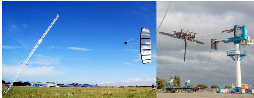
Fig. 18.3 Two groups experimenting with towers/masts. Left: TU Delft’s demonstrator, provided by Roland Schmehl. Right: Makani Power’s/Google’s 600 kW prototype [25], reprinted with permission of Fort Felker
