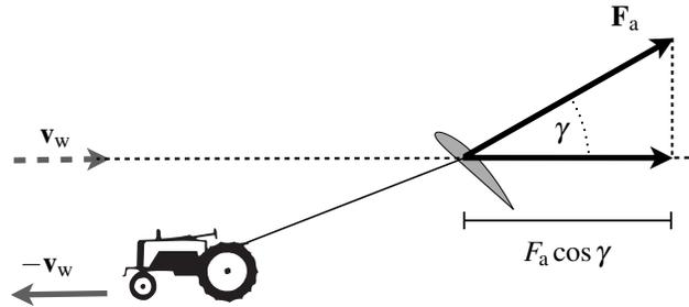
**Fig. 1.4** Thought experiment from the proof of Lemma 1.1. A tractor moving at speed  $v_w$  and pulling a wing through air at rest performs a mechanical power of  $v_w F_a \cos \gamma$ . Conversely, if the air moves and the tractor is at rest, the same amount of power is extracted from the relative motion of the air with respect to the ground. It constitutes the power  $P_{\text{wind}}$  lost by the wind field due to the presence of the wing.
