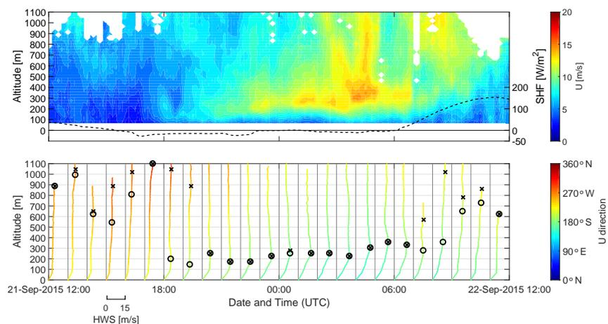
Figure 1: Visualization of measured 10-minute mean wind speed and wind direction of a 24 hour period between September 11-12th 2015. The top sub-figure shows the LiDAR-measured wind speed and WRF calculated SHF(dashed line). The bottom figure shows each hours wind speed profile colored according to wind direction. X marks the altitude of highest wind speed and O denotes optimal operating altitude according to the idealized traction power approximation.
