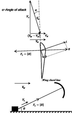
Fig5: Aerodynamic Forces during crosswind flight [1, 5]
