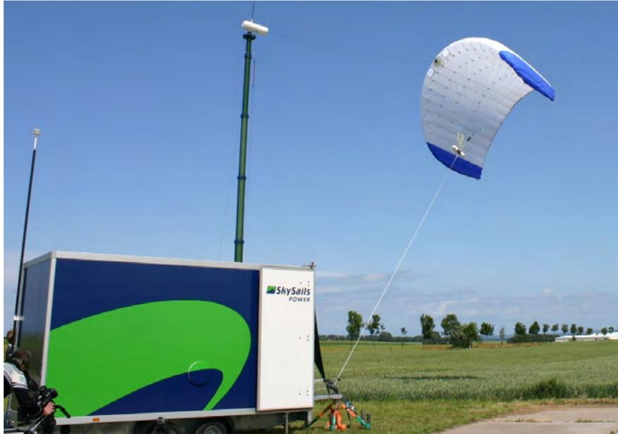
**Fig. 20.11** SkySails Power functional model
