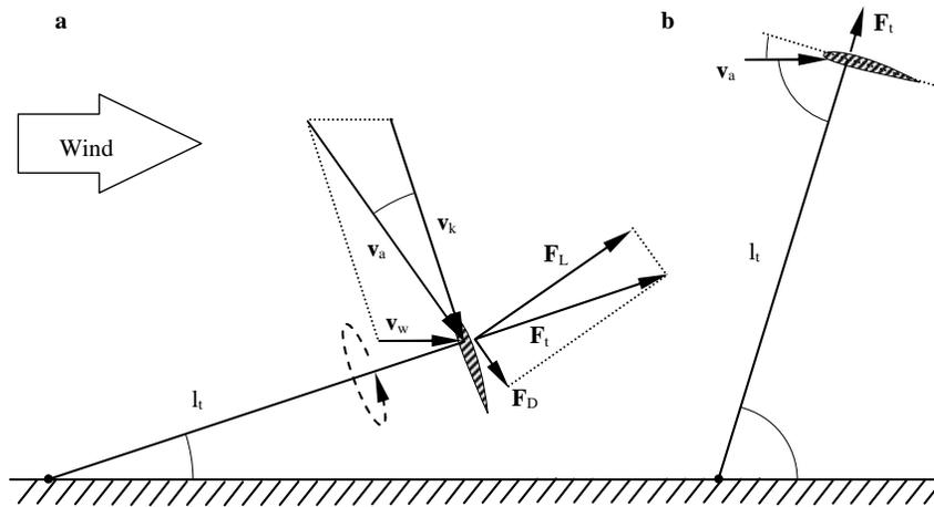
**Fig. 20.6** a Force and velocity vectors at a kite in a continuous loop, b kite in a static position
