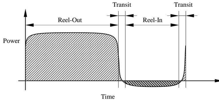
**Fig. 20.10** Idealized power profile for one pumping mode cycle
