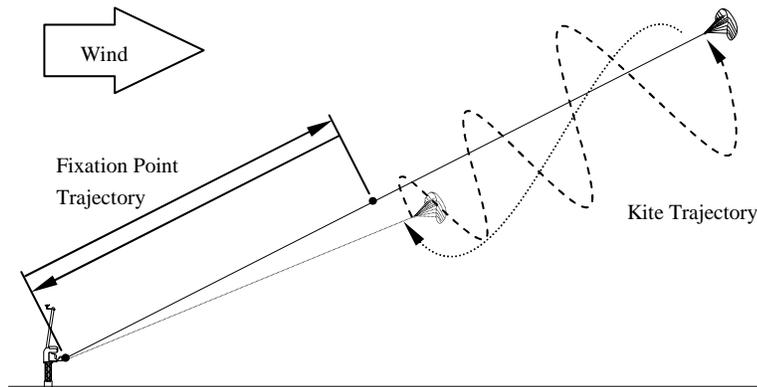
**Fig. 20.9** Kite and fixation point trajectories for the pumping mode energy kite
