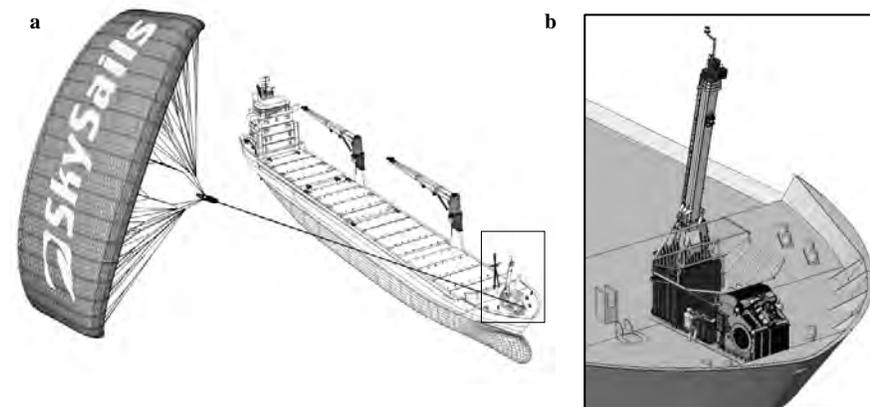
**Fig. 20.3** **a** CAD drawing of multipurpose vessel with SkySails system SKS C 320, **b** CAD image of forecastle installation
