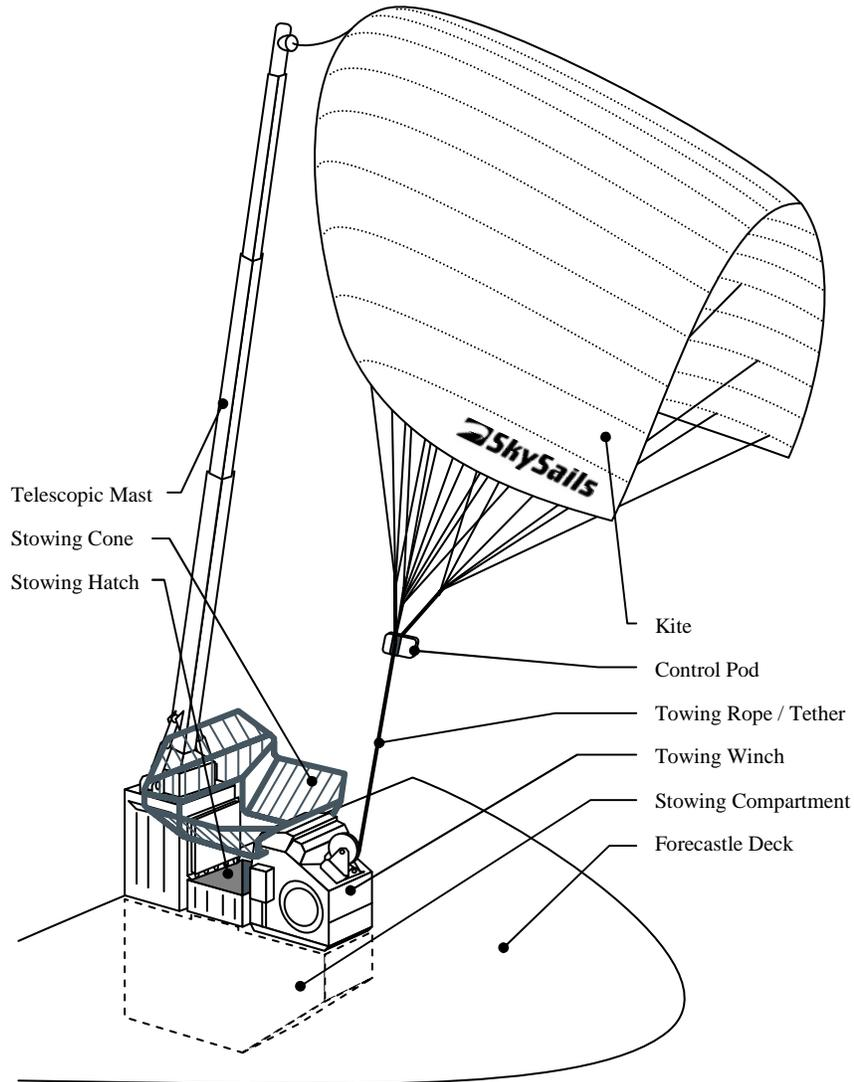
**Fig. 20.5** SkySails Marine Launch and Retrieval System
