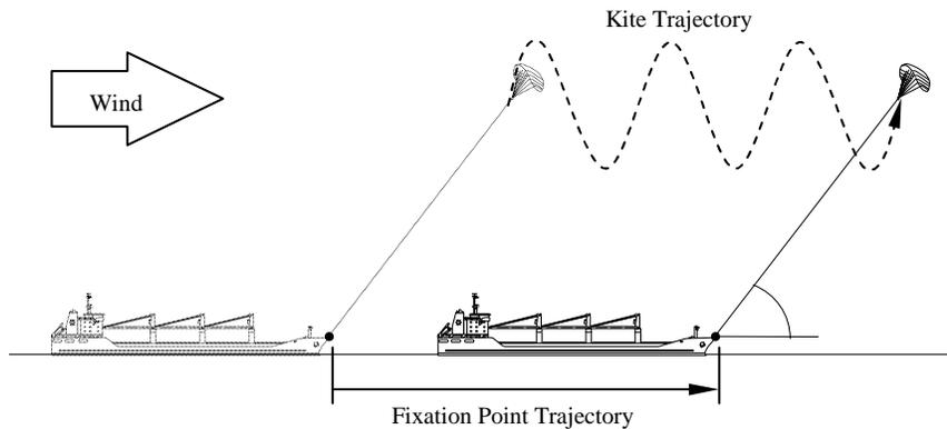
**Fig. 20.7** Kite and fixation point trajectories in the ship propulsion application
