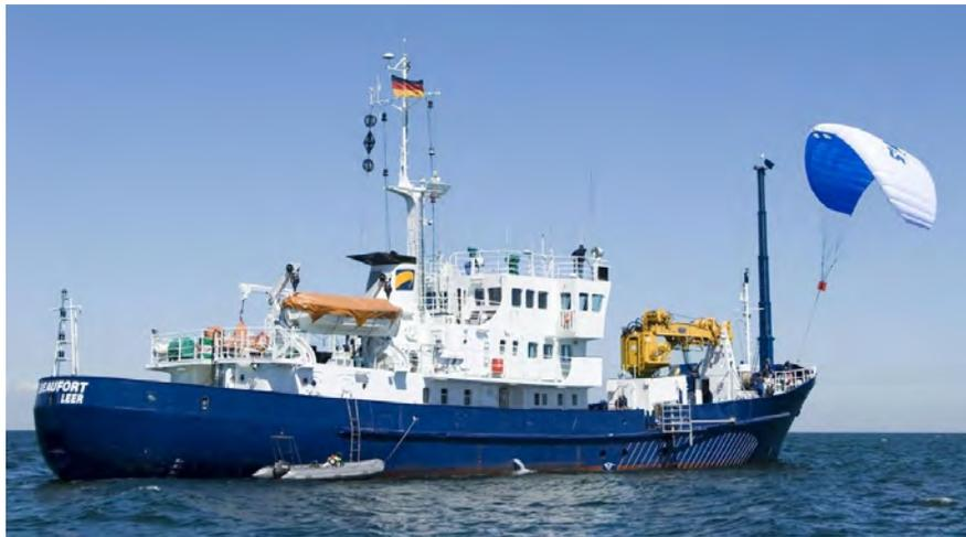
**Fig. 20.1** Research vessel MV “Beaufort” during launch of the towing kite
