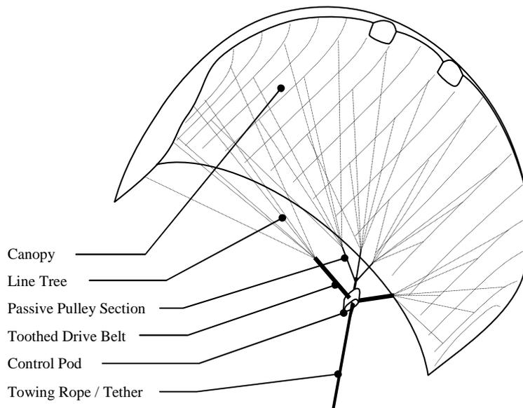
**Fig. 20.4** SkySails kite and control pod
