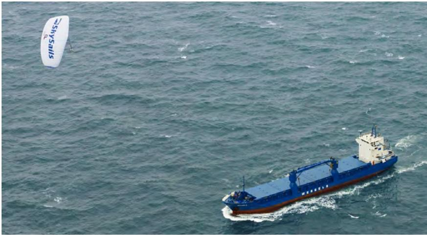
**Fig. 20.2** Pilot customer vessel MV "Michael A." with towing kite in operation
