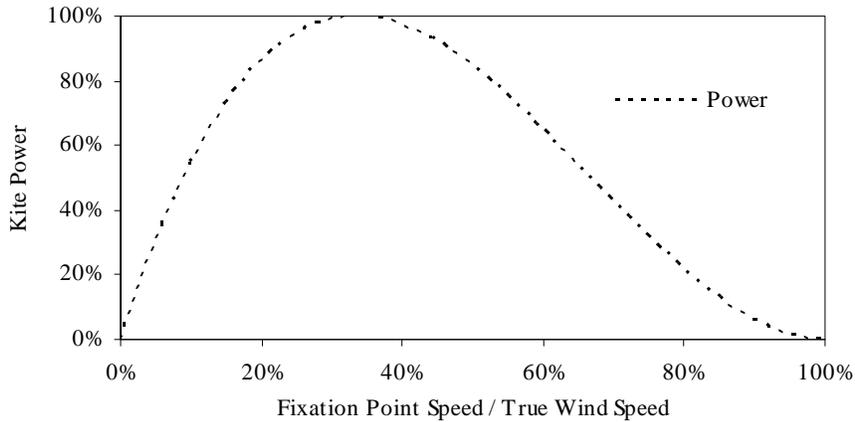
**Fig. 20.8** Normalized kite power output dependent on the ratio of fixation point speed and true wind speed
