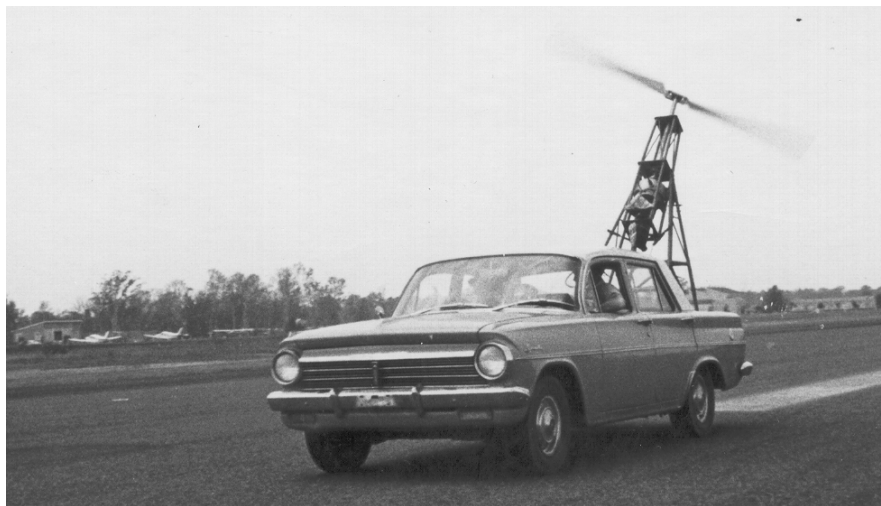
Fig. 23.4 Test setup for rotor at incident angle
