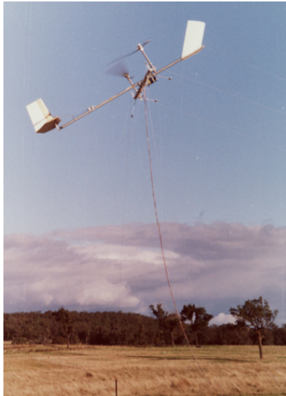
Fig. 23.7 The Gyromill Mk2 was equipped with twin, single bladed, counterweighted rotors of solidity 2.2% and a diameter of 3.65 m. The total mass of the craft was 29 kg. Again no cyclic pitch capability was employed. Thus in hover and wind it was found necessary to use three parallel tethers to maintain craft attitude. These three tethers were used in all tests, but the craft was difficult to control particularly in low winds. Two tethers were attached near the rotor thrust lines while the third tether was attached well forward on the forward pointing boom
