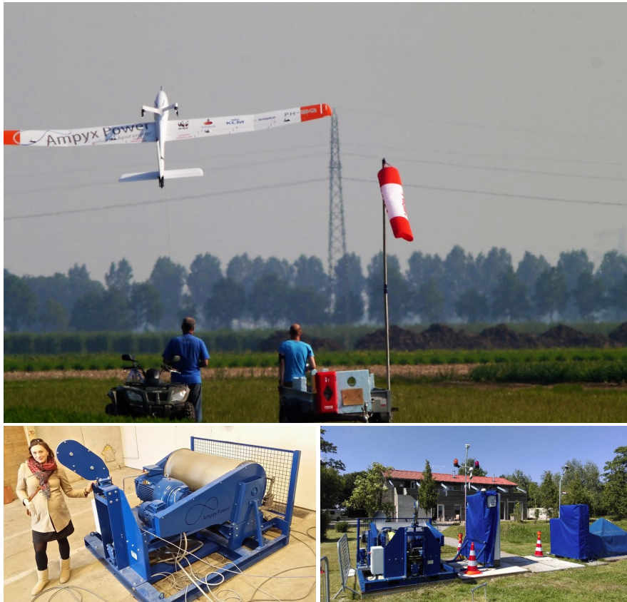
Fig. 26.4 AP-2A aircraft, 90 kW generator and control center
